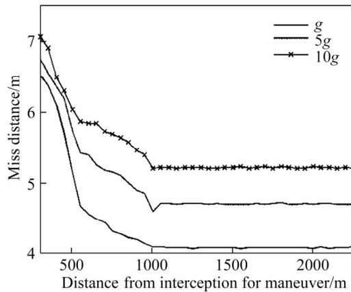
Figure 6 Sensitivity to target maneuvers for DI-TSMC
