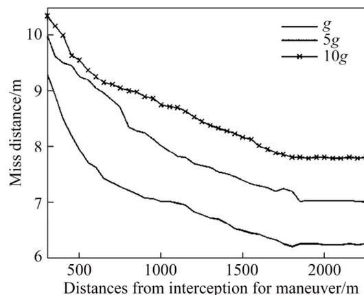
Figure 7 Sensitivity to target maneuvers for ANTSMC
